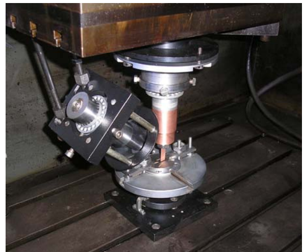
Figure 11 Photo of the equipment mounted on ELER 01 Romanian EDM installation
