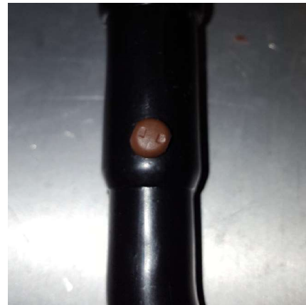
Figure 11. Dissimilar steel-plastic joint without defect
