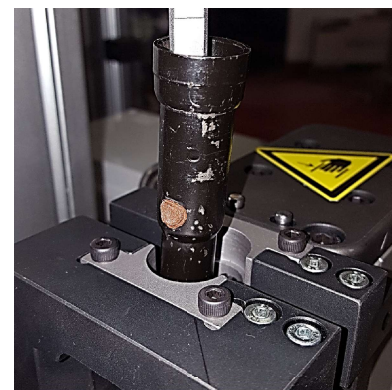
Figure 12. Defective dissimilar steel - plastic joint
