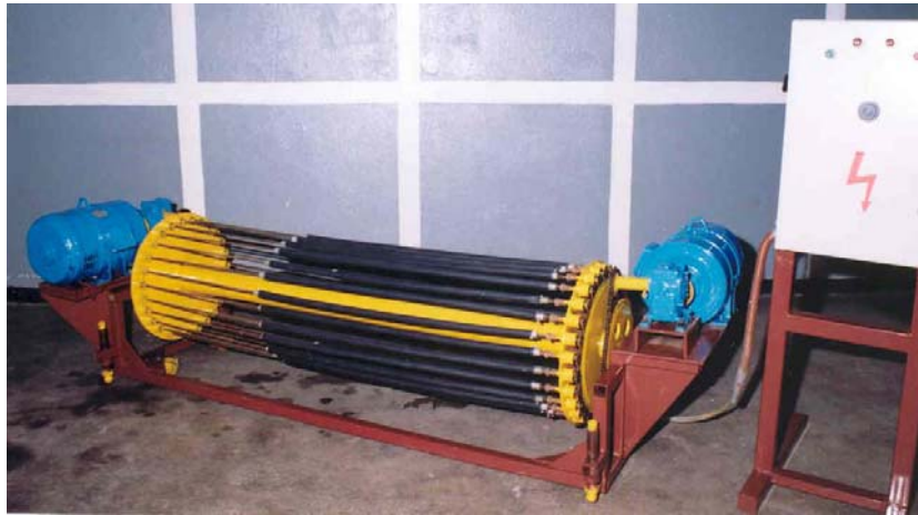
Fig. 4. Complex equipment for irradiation with electron beam of heat shrinkable tubes.
