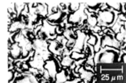
Fig. 2. Surface microgeometry at usual finishing ( R_a=1 \mu\text{m} )
