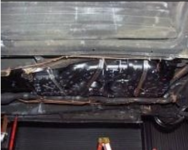
Figure 3. The fuel tank installed for test
