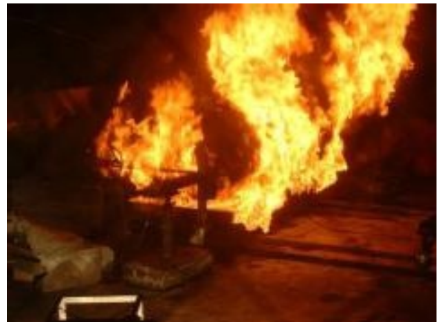
Figure 7. Running the phase 2 of testing the fuel tank.
