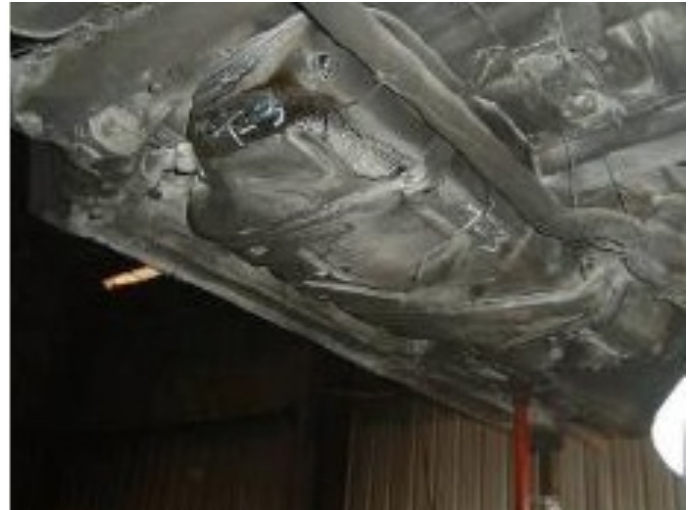
Figure 12. The fuel tank that did meet the requirements regarding fire resistance test.
