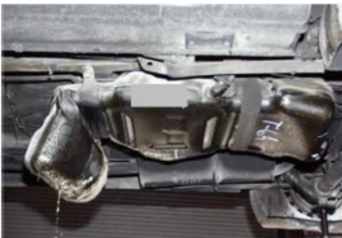
Figure 11. The fuel tank that did not meet the requirements regarding the fire resistance test.
