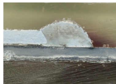
Figure 3. Macrostructure of braze-welded sample 0, the central point
