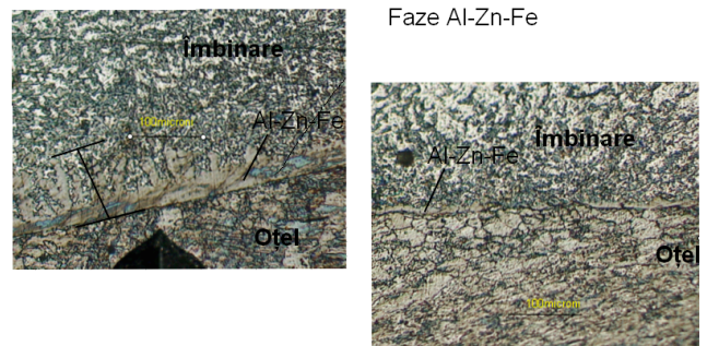
Figure 7. The diffusion layer of zinc measurement mode
