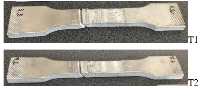
Figure 6. Processed material specimens, tensile tested
