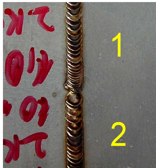
Fig. 6. Overlap welding with pulse duration: 1) \tau_H=8ms ; 2) \tau_H=10ms .
