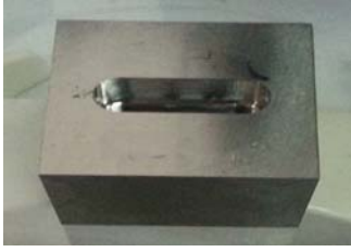
Figure 8. Cavity shape obtained through milling
