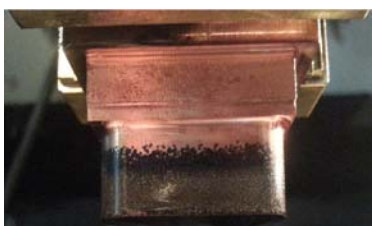
Figure 9. Cooper profiled electrode used in experiment
