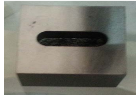
Figure 11. Cavity shape obtained through EDM
