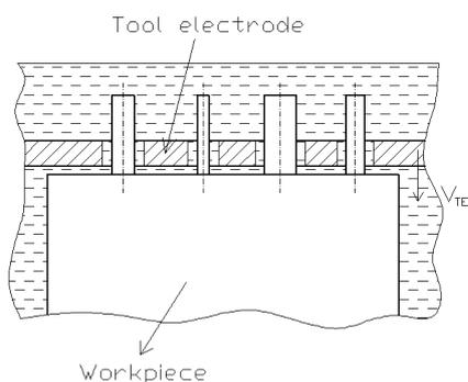
**Figure 3.** Machining scheme applied in order to obtain small diameter cylindrical surfaces by means of a plate tool electrode
