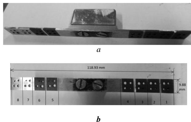
**Figure 4.** Tool electrode used in the experimental research (a) and the aspect of the tool electrode active surface after the electrical discharge machining process (b)
