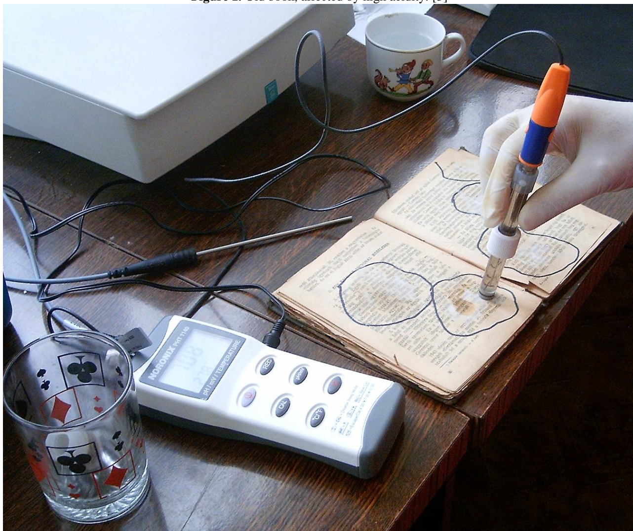
Figure 2. pH measurement for the treated old book. [3]
