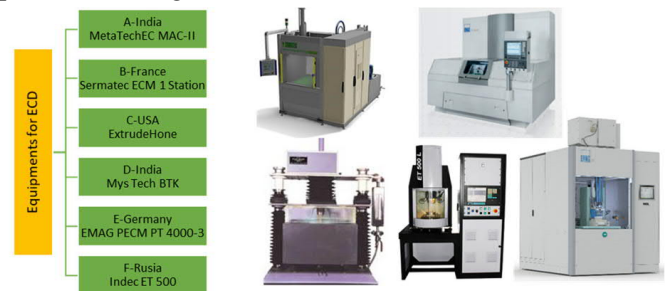
Figure 6. Equipments for Electrochemical deburring available on the market [13], [14], [15], [16]
