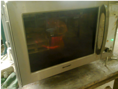
Figure 1. The experimental 0.8 kW-microwave oven
