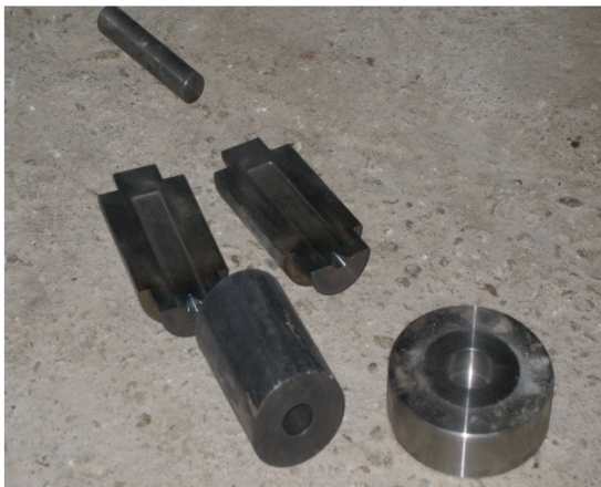
Figure 3. Injection heating matrix components
