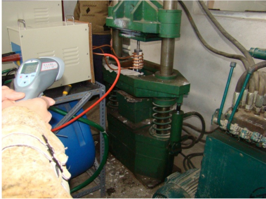
Figure 5. Experimental manufacturing line by thixotropy and injection in matrix
