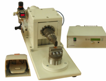
Figure 5. Specialized hybrid equipment for electric pressure and ultrasonic welding
