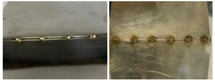
Figure 3. – Temporarily welded sheets (weld points), corner, 1 mm thick, steel 1.4301(304), (A1-A4)
