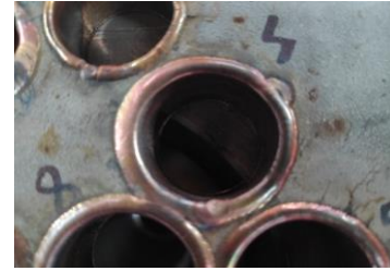
Figure 10. Result of the test piece heat exchanger welding for the reference 4 copper pipe
