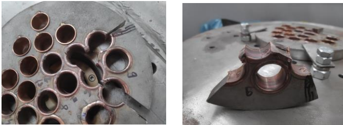
Figure 12. Cutting of the heat exchanger test piece
