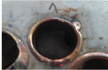
Figure 8. Result of the test piece heat exchanger welding for the reference 1 copper pipe
