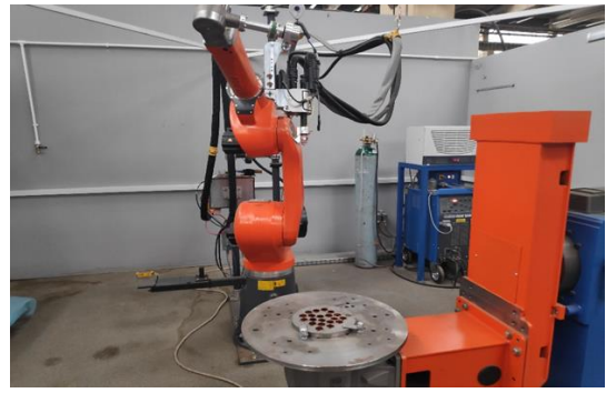
Figure 3. Setting up the intermediary point 10 for the robotic GTAW system
