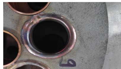
Figure 11. Robotic welding of the reference 9 copper pipe within the heat exchanger test piece
