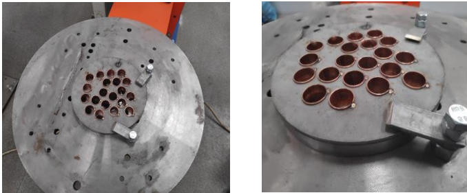
Figure 2. The test piece used for performing the GTAW welding of the copper pipes with the robotic system
