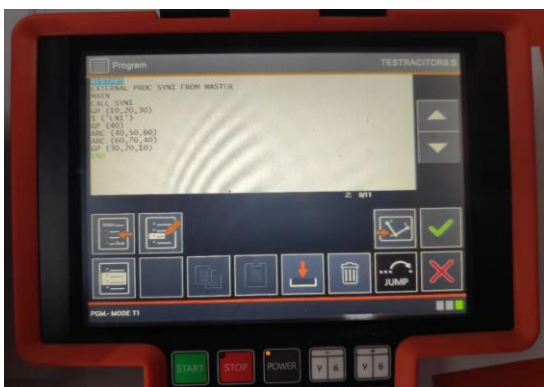
Figure 6. The console developed software program for welding each copper pipe to the test piece
