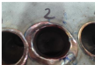
Figure 9. Result of the test piece heat exchanger welding for the copper pipe with reference 2
