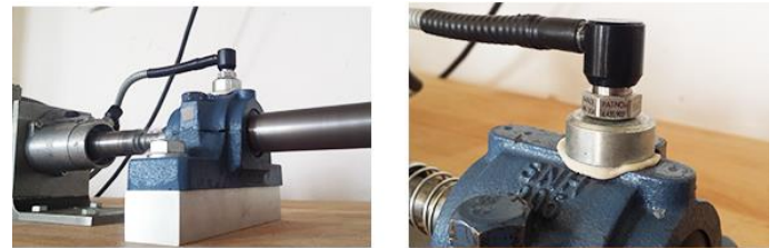
Figure 3. Position of sensor type PCB 607A11 with mounting detail on the bearing housing
