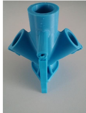
Figure 6. Intake gallery - PLA material 3D printed
