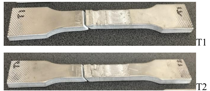
Figure 6. Processed material specimens, tensile tested
