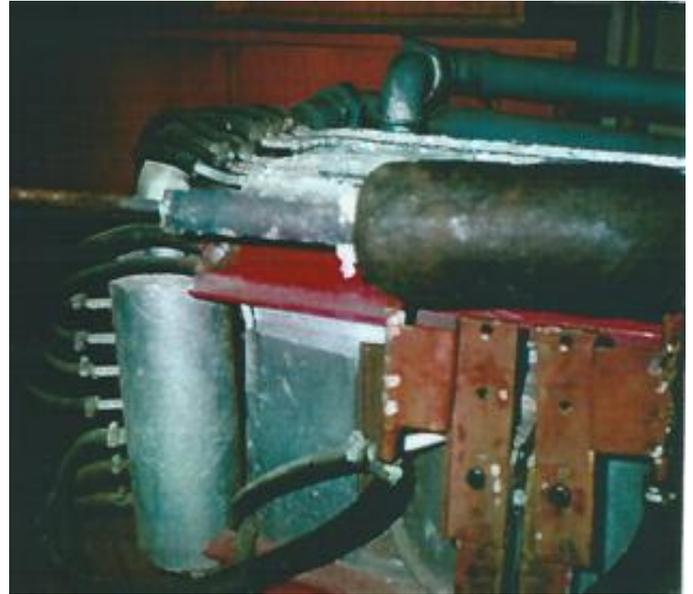
**Fig.15** The heating process with the double layers inductor, and magnetodielectric field concentrator
