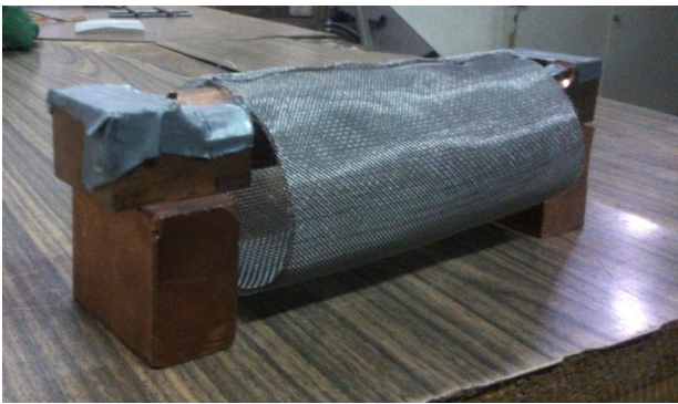
Figure 9. Positioning of the filter for welding.
