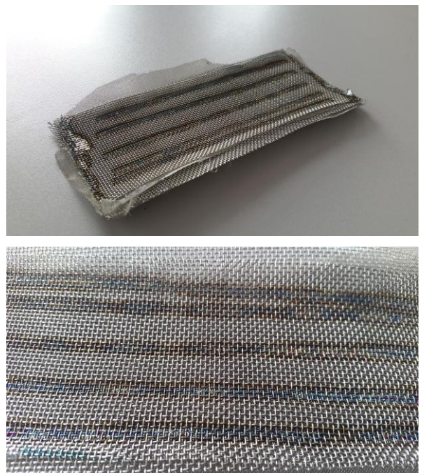
Figure 12. Aspect of pressure welds (down - detail).
