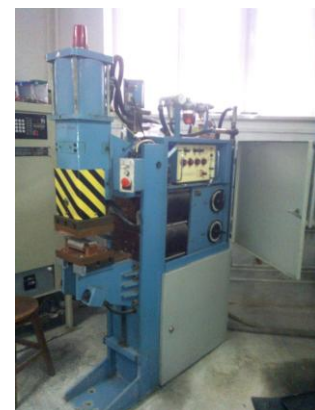
Figure 7. ZGB-80 projection welding machine.
