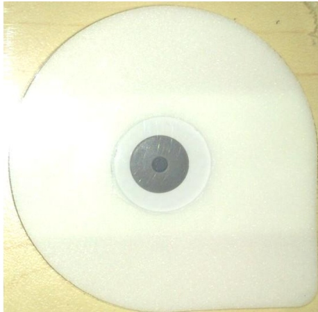
Figure 3. Example of Ag/AgCl electrode used in recording
