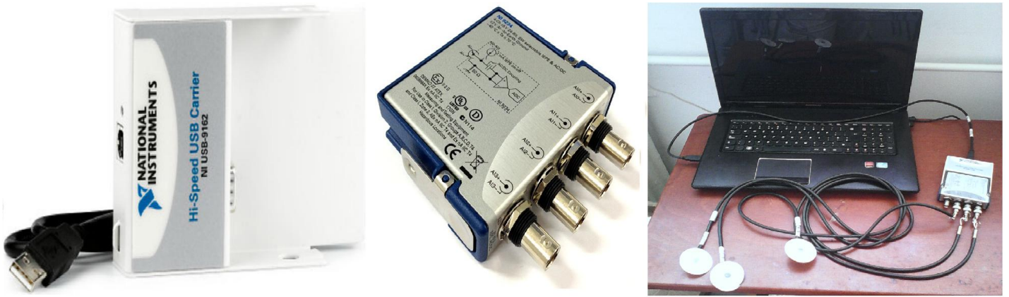
Figure 2. The NI-USB 9162 High Speed USB Carrier (left); The NI-9234 ADC (middle); The whole recording system (right)
