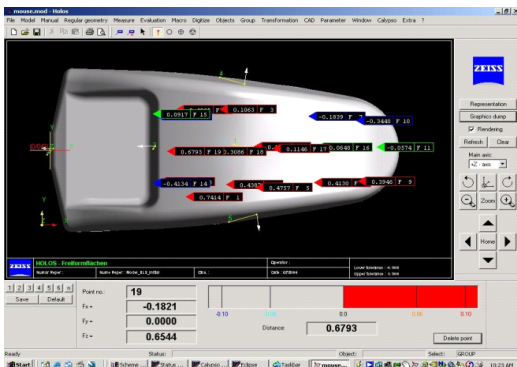
Figure 8. Graphic representation of results obtained by measurement of part manufacturing by SLS process
