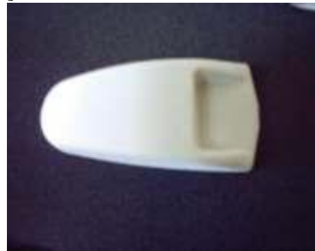
Figure 1. The SLS model, obtained by selective laser sintering process
