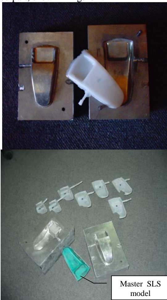
Figure 4. Removed the injection part from the mould made through the process of spraying molten metal
