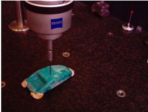
Figure 7. Sequence performed during the measurement of the SLS part on the machine prototype ZEISS ECLIPSE 500
