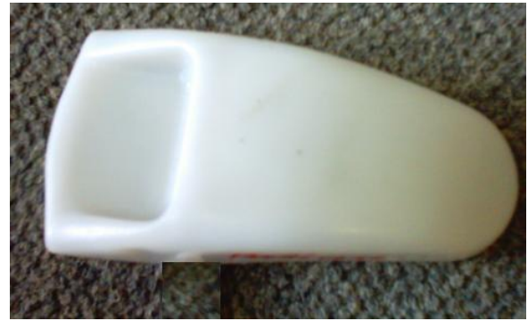
Figure 5. The polypropylene part made by injection into the mould obtained by spraying molten metal
