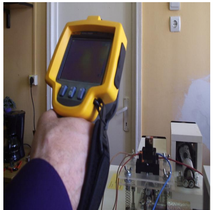
Figure 3. Measuring the temperature on the contacts of the relays without vibrations
