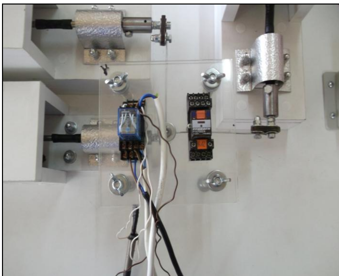
Figure 1. Testing the electrical relays to vibrations. On the left-hand side one can see the Omron electrical relay, and on the right-hand side, the Schrack electrical relay
