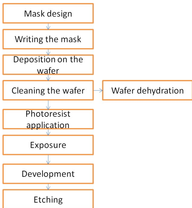
Figure 1. The steps of the photolithography process
