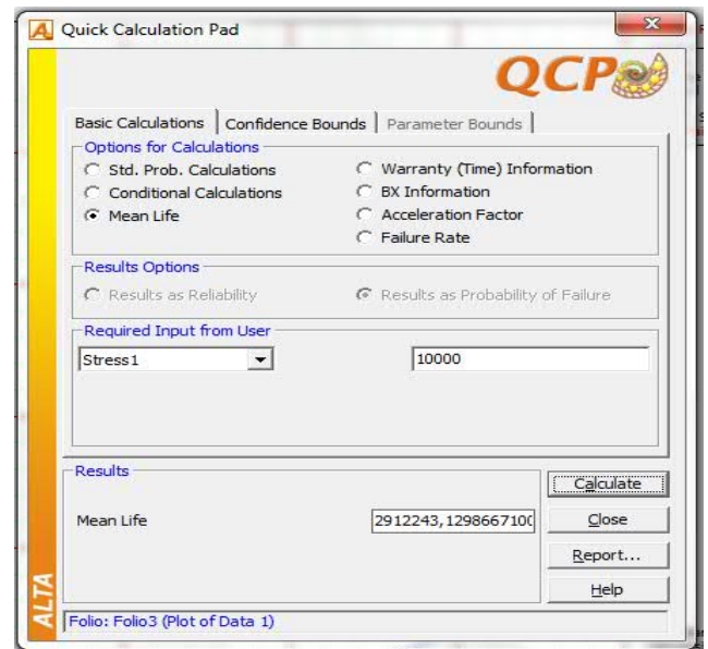
Figure 15. The determination of the number of cycles to failure of the blades in normal testing conditions
