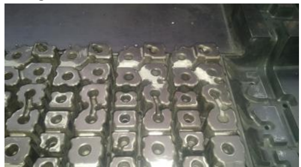
Figure 10. Minus of material on the mold.
