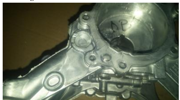
Figure 11. Burrs and shrinkage on the parts(defect)
