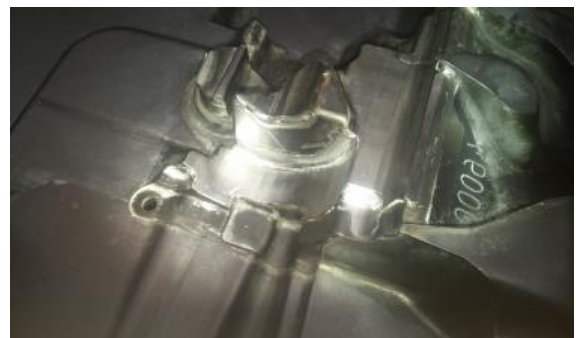
Figure 3. Milled surface on the mold
