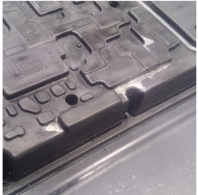
Figure 6. Polishing surface of the mold.
