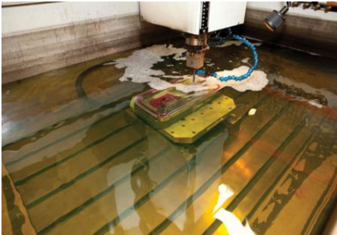
Figure 4. Electrical discharge (EDM) used by die casting mold
