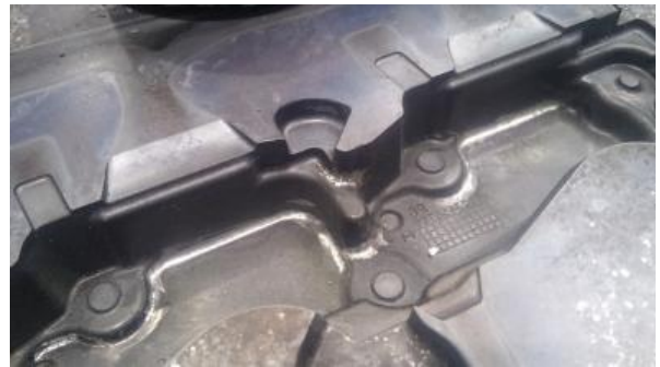
Figure 9. Worn, break and cracks on the mold.
