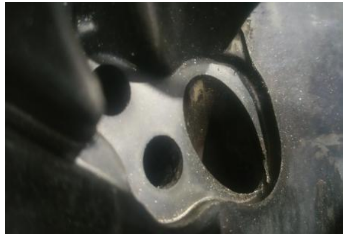
Figure 14. Broken corner on the mould (before reconditioning)
