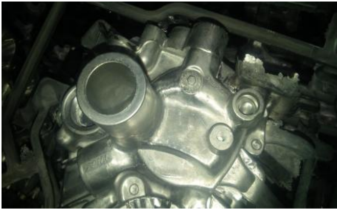
Figure 13. Lamination and Cold Flow on the parts(rework by Sand Blasting).
