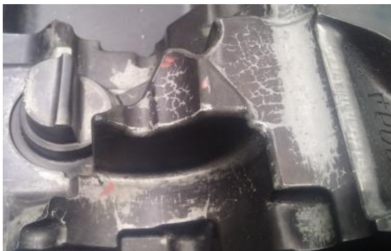
Figure 1. Cracks on die casting mold
