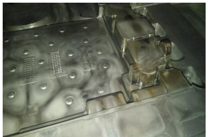
Figure 7. The die casting mould after the reconditioning.
