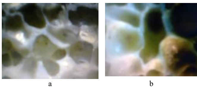
Figure 3. Microstructural images of the cross sections of the glass-ceramic foam samples. a - sample 3; b – sample 4.
