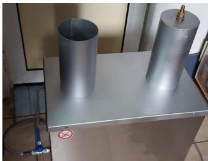
Figure 14. Ultrasonic cavitation filtering system
