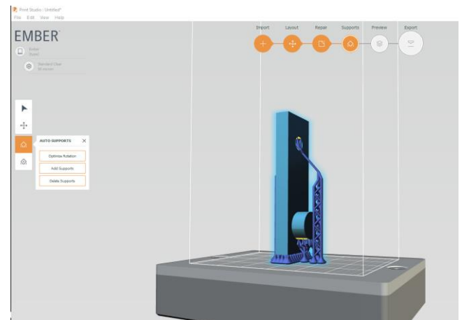
Figure 4. Position and supports for generated probe for Ember printer with Photo Studio program
