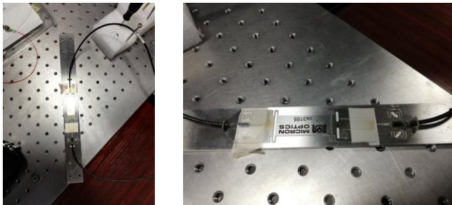
Fig. 7. Mounting optical fiber on metallic structure
