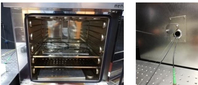
Fig. 8. Arrangement of optical fibers in Memmert UE300
