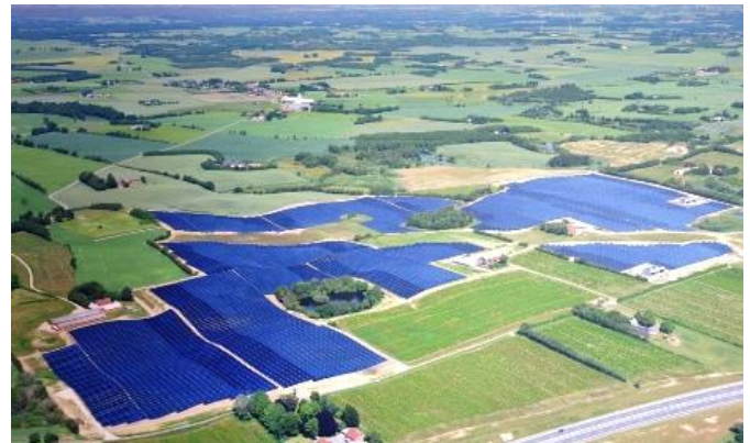
Figure 17: World's largest solar district heating plant in operation in 2018 (110 MW th ) in Silkeborg, Denmark.
