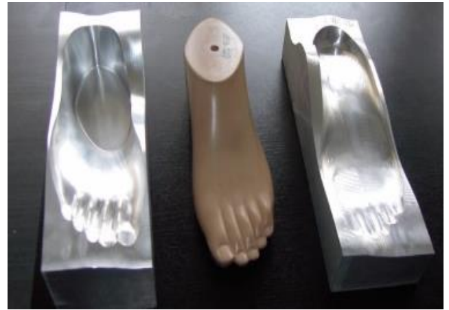
Figure 6 Manufacturing of SACH using injection mold
