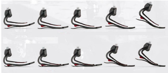
Figure 4 THRIVE - response with no extra load (upper), response with extra load (bottom) [3]
