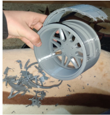
Figure 10. Left the printed rim and right the process of remove the supports
