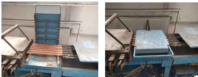
Figure 5. Fixing and soldering of the exchanger element subassembly
