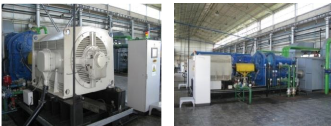
Figure 1. View of electrically driven centrifugal air compressor CCAE [1]
