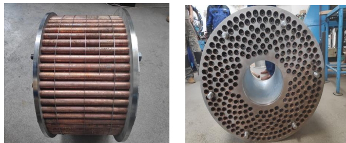
Figure 2. Side and frontal view of the heat exchanger assembly
