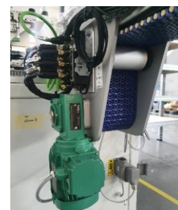
Figure 5. Two geared motors
