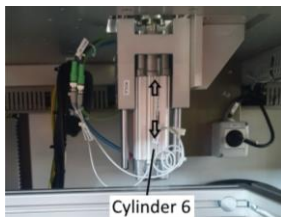
Figure 13. Solenoid valve corresponding to cylinder 6
