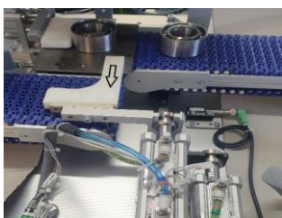
Figure 14. Sensor confirms the new bearing position
