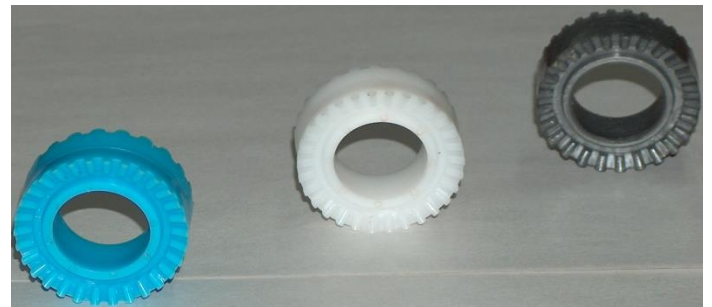
Figure 5. Satellite gear wheels cast from different plastic materials.
