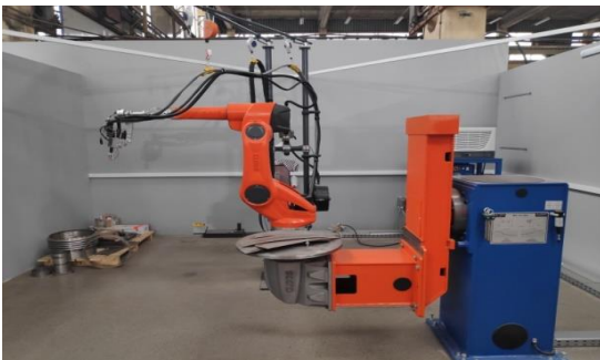
Figure 1. The work cell for the 8 axis welding robotic system
