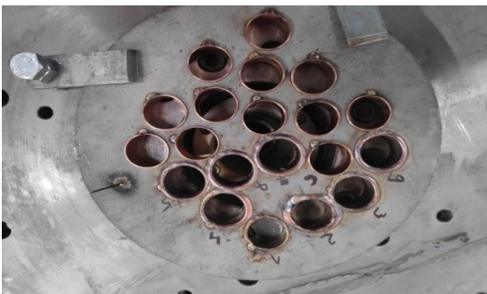
Figure 3. Specimens obtained from the robotic welding process on the test piece [6]
