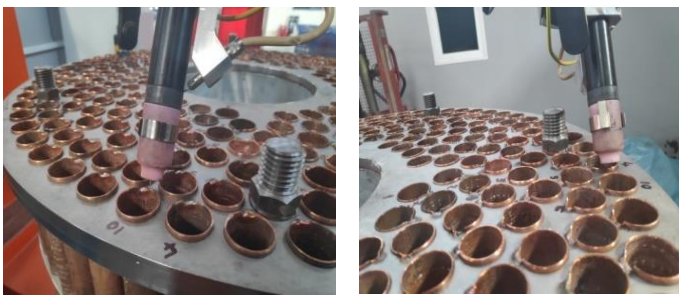
Figure 7. The first two points on the arc length of a pipe for the software program of the robotic system
