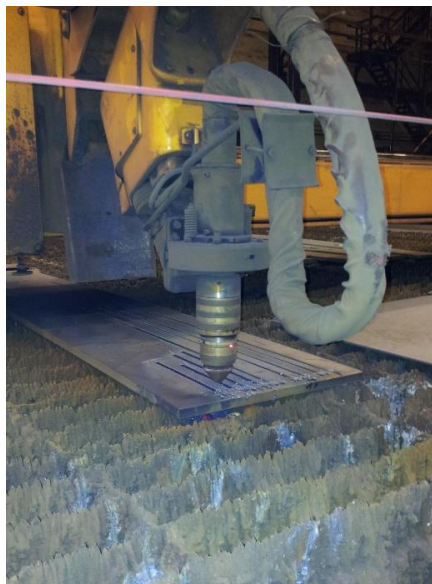
Figure 1. Detail of the HiFocus 280i plasma head Table 1. Basic material properties of type S355J2C
