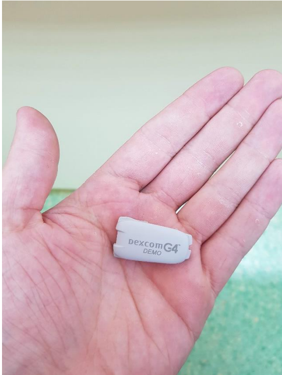
Figure 3 – Dexcom G4 continuous glucose monitoring device used in the clinical research for patients with Diabetes Mellitus
