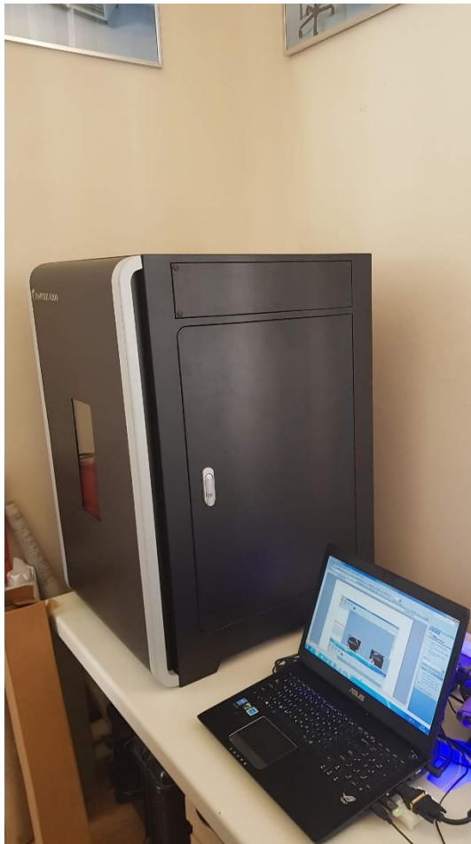
Figure.1 – Rapid prototyping cell – Inspire S200 3D printer and a laptop used for the computer aided design software and the manipulation of the 3D printer
