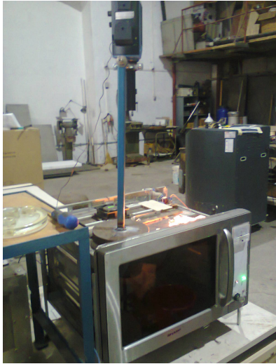
Figure 1. Image of the microwave installation used in the experiment
