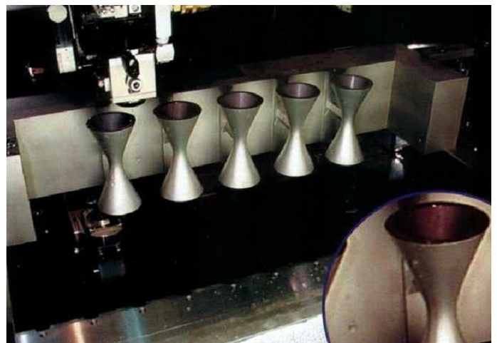
Figure 2. Hyperboloid surfaces processed using wire electrical discharge machining
