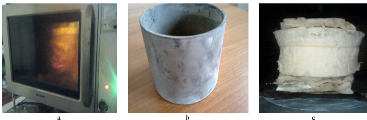
Figure 1. Pictures of the wave oven and its components used in experiment a – 800 W-wave oven; b – ceramic tube; c – heat protection of the tube and its lid.
