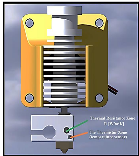
Figure 7. The housing of the thermal resistance and the temperature sensor
