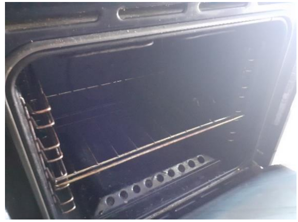
Figure 1. Appearance of 1.5 kW-laboratory electric heating oven
