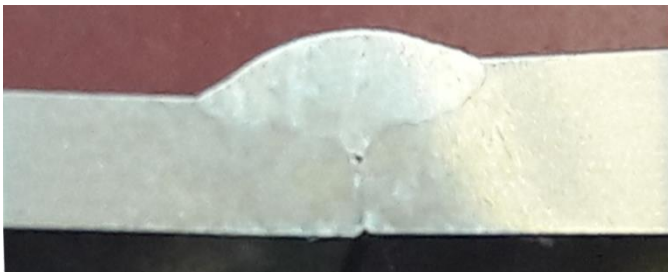
Figure 2. Metallographic image of the first sample reconditioned by welding
