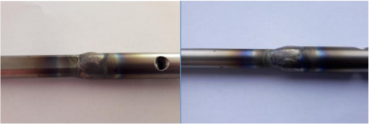
Figure 5. The welded seam obtained through the second welding reconditioning technology
