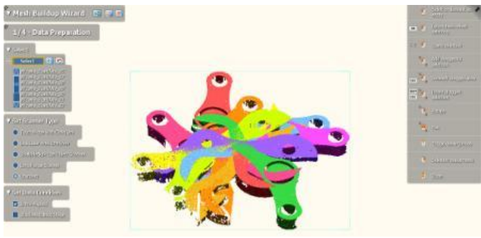
Figure 8. Scanned data imported into the reverse engineering application
