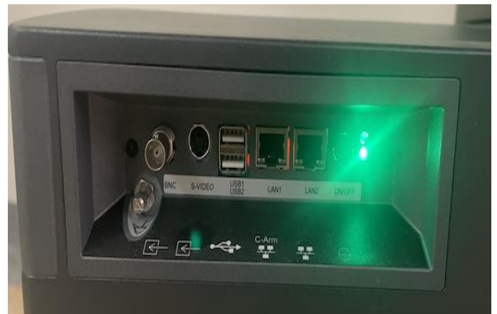
Figure 2. Figure 1 Input-output slots and ports in a neuronavigation system (Source: Authors' own research contribution)
