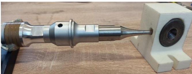
Figure 6. Schematic of the ultrasonic activation of the die
